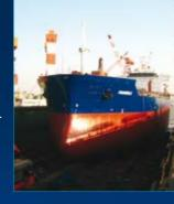
This is the first vessel ever to be coated with polysiloxane technology from Jotun Coatings. The product was chosen as a test bed for gauging the improved performance properties over existing two-pack topcoats. With improved weathering capability and with excellent opacity and gloss retention, Hardtop PS5 provides an owner with a far more versatile coating in the long term than any other two-pack generic topcoat used to date.
