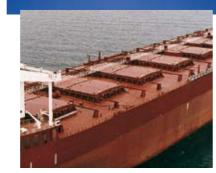
A zinc epoxy primer in combination with Hardtop Flexi is often chosen to protect decks and hatches. Now a 50 micron (min) coat of Barrier followed by a 150 micron (min) coat of Hardtop Flexi will provide good lasting protection of these impact prone areas.
