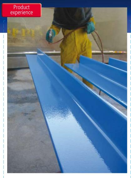
Hardtop XP has been tested with several applicators. The high dry film thick thickness tolerance of Hardtop XP has been especially appreciated by painters. It is not technically possible to achieve an even dry film thickness on the different angles and corners of many industrial objects, being aware that Hardtop XP is one of the most tolerant products in its category adds to the painter's confidence.
